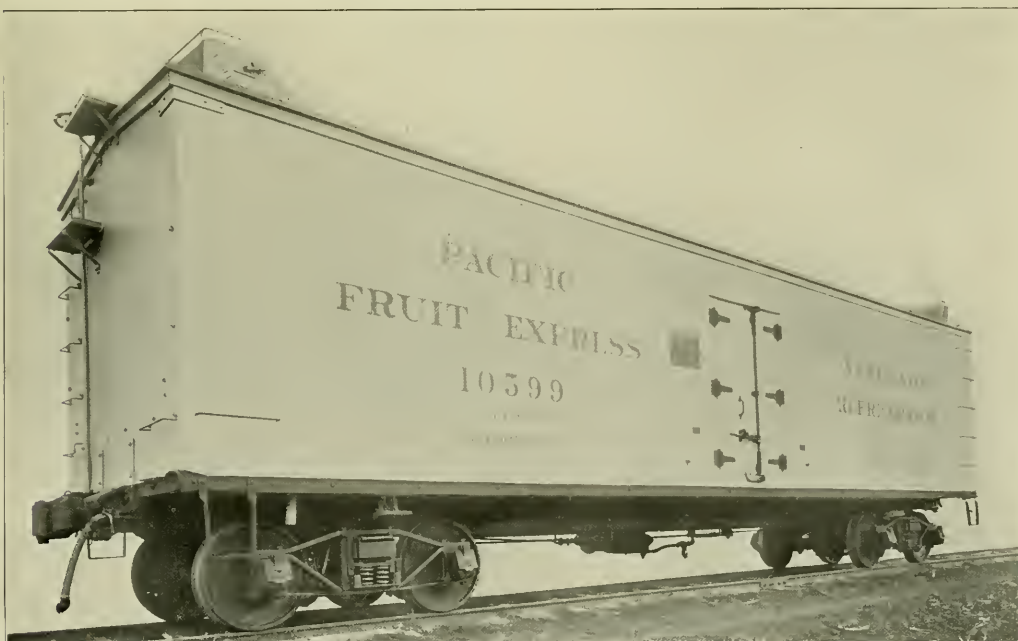
Refrigerator Car with Bettendorf Steel Underframe.
